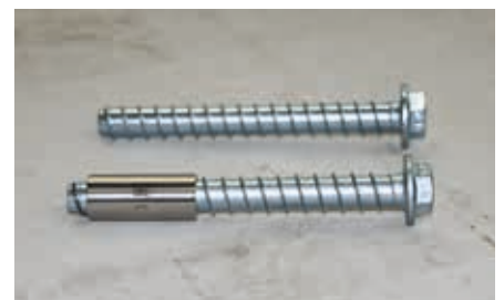
Anchor fits through the gauge - reuse is not possible
