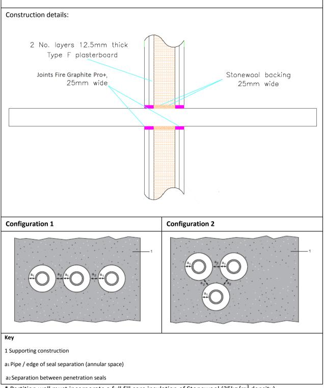
\* Partition wall must incorporate a full fill core insulation of Stonewool (35kg/m<sup>3</sup> density)
