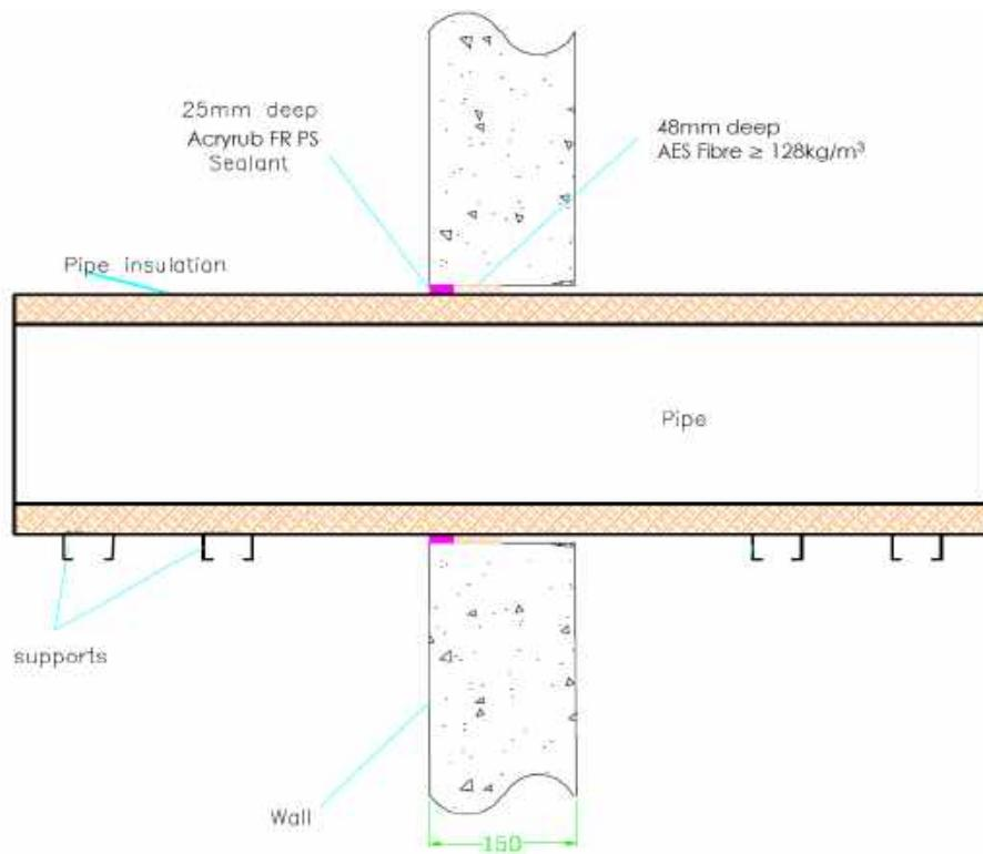
**A.1.5.1 Single side penetration seal with pipes**
