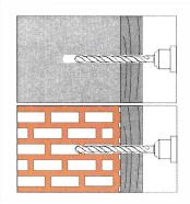
Drill the hole considering the drilling method and clean the hole of drilling dust.
