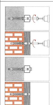
Screw-in the special screw until the head of the screw touches the sleeve; the anchor is correct mounted, if there is no turn-through of the plastic sleeve in the drill hole and if slightly move on turning of the screw is impossible.
