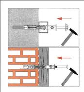
Insert the plastic sleeve and special screw into the hole through the fixture by slight hammer blows.
