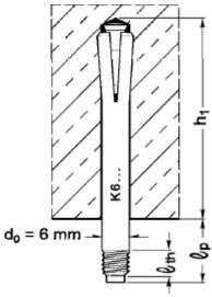
$L_{th}-$  Length of connection thread  $L_{p}-$  Length of protrusion
