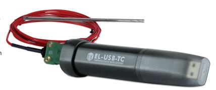
This standalone data logger measures and stores more than 32,000 temperature readings from a J, K or T-type thermocouple at a resolution of 0.5°C (1°F). It comes supplied with a K-type thermocouple capable of measuring from 0 to +200°C (+32 to +392°F).
